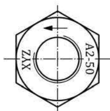
Figure 8 — Example of marking for left-hand thread
